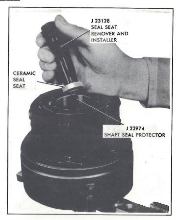
9. Using tool J-9392 engage tangs on tool with those on seal by rotating tool clockwise and pressing down. Seal can then be removed.
