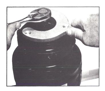
4. Screw hub puller (J-9401) into hub. Hold body of puller with a wrench, and tighten center screw of puller until drive plate, hub and key can be removed.
