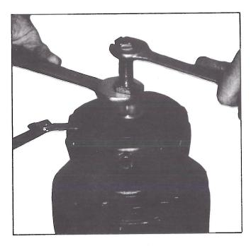
NOTE: Ensure hub key remains in place while pressing hub on shaft.
