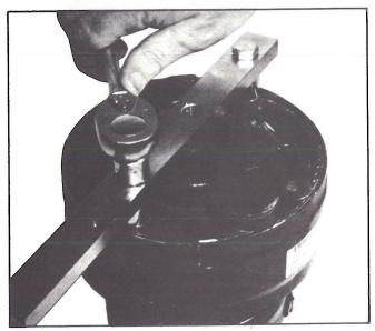
3. Remove the clutch drive plate and hub by first removing the 9/16" nut on the compressor shaft (J-9399 Thin Wall Socket and J-25030 Hub Holding Tool).
