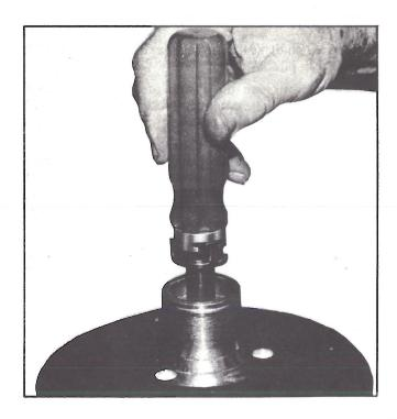
10. Using tool J-9553, or small probe, remove seal seat "O" ring.
