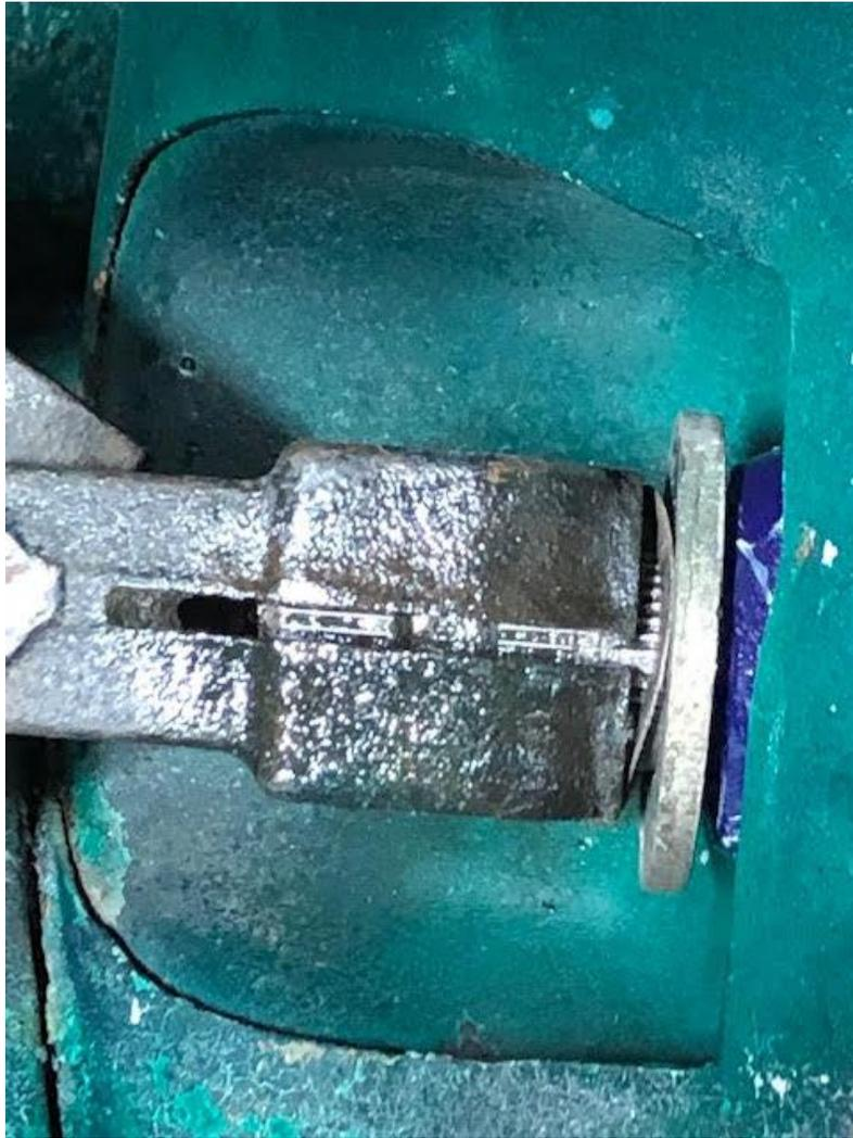
Inside the car, slide the “U” clamp back up to the main bracket and keep in mind that part of the column is also slotted. So the clamp only goes on one way.
