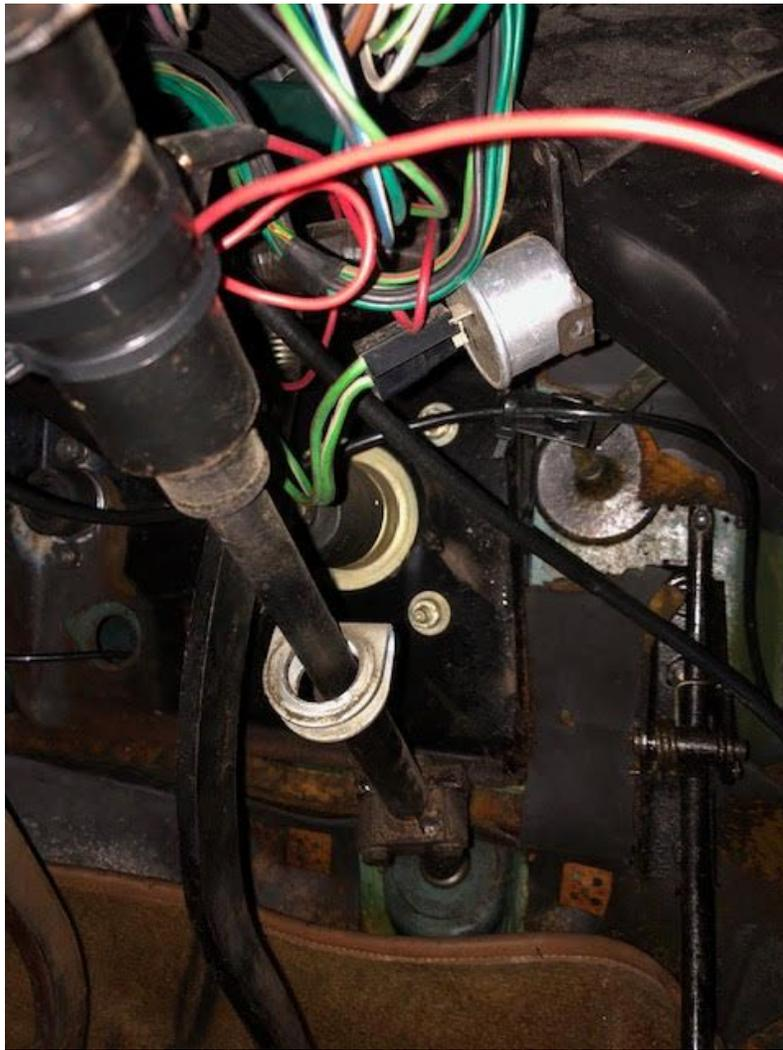
Sit in the driver seat and press your knee under the steering wheel and hands at 10 and 2 and rotate pressure back and forth until the column comes out of the knuckle and through the firewall. There is a large washer and small spring washer in between the knuckle and firewall that will fall down.
