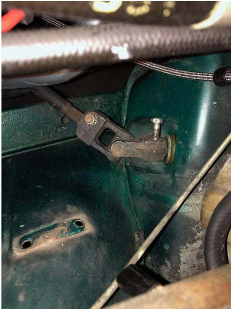
Inside the car, remove the nut and bolt holding the “U” clamp on, on the upper side of the column just after the main bracket and slide the clamp down and out of the way.
