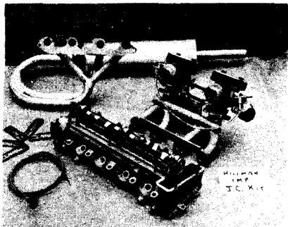
Above: twin 1½ ins. SUs as supplied by Nerus for the Imp, other well known tuners sell this type of conversion for about £30 and results are generally good. Below: HS6s (1¾ ins.) as fitted to the MGC; its sister the MGB uses the visually similar 1½ ins. twin HS4 carbs.
