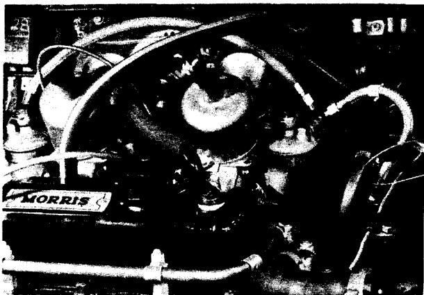
A works Mini Cooper S: within the engine department lurk these twin 1½ ins. SUs in place of the standard 1½ ins. carbs. Note the carb bellmouths and the re-routed oil breather pipe all very neatly done.
