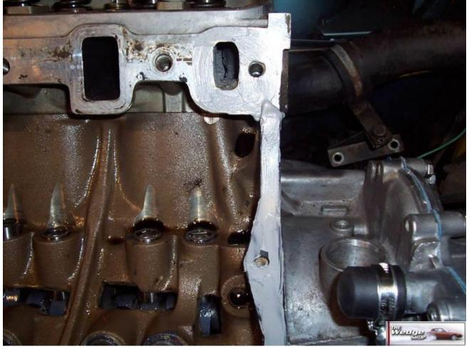
Then apply a liberal amount of sealant to the top of the end seals like so. You can never have too much sealant, you can always just wipe off the excess after you are done bolting it down.
