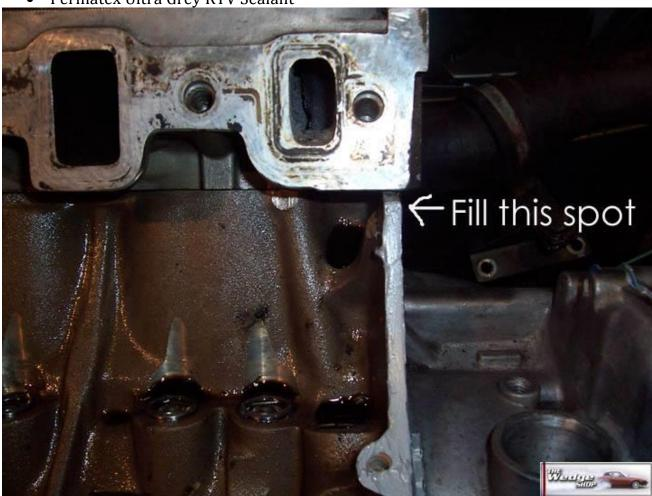
As seen in the first picture, we show you how important it is to seal up the space between the head & the block with sealant. The first photo shows the space unfilled. While the second photo shows the space filled with sealant.
