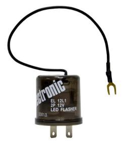
For the flasher, if you are installing these on a TR8, when looking at the flasher with the middle tab on the top, hook the green brown to the right prong and the green light pink to the left prong.
