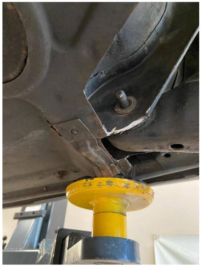
Paint the bare metal areas before installing the braces
